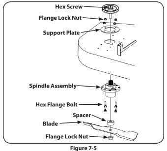
Reverse the process to install the spindle assembly.
